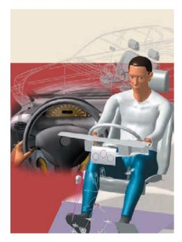
During the course of extensive experiments, research institutes have analyzed the postures and behavior of persons in a vehicle. Thanks to the embedding of the acquired information into the RAMSIS databases, the posture of the driver can be simulated and realistic forecasts with regard to future room and operating conditions within the vehicle can be made.
