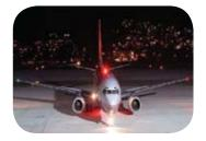
**EXTERIOR LIGHTING** Navigation, positional, anti-collision, aircraft recognition, formation, taxiing and landing lights
